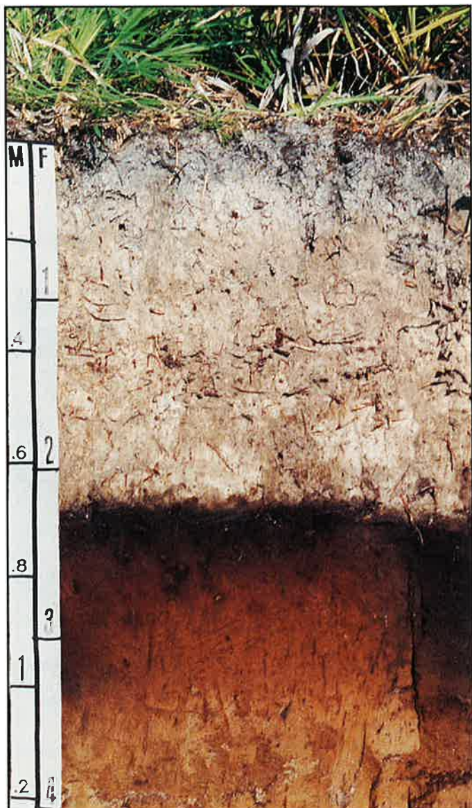
Figure 2. Myakka fine sand profile. A six-inch surface layer of friable gray fine sand, a twenty-inch subsurface layer of light gray fine sand, a six-inch subsoil of dark reddish brown fine sand organic stained layer, with a brown and yellowish brown fine sand substratum.
